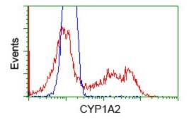
HEK293T cells transfected with either pCMV6-ENTRY CYP1A2 ([RC221636]) (Red) or empty vector control plasmid (Blue) were immunostained with anti-CYP1A2 mouse monoclonal (TA501172), and then analyzed by flow cytometry.
